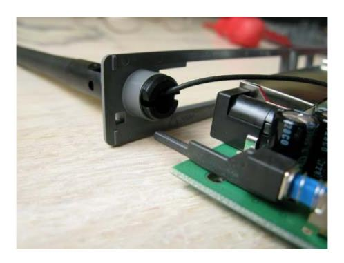
Now, remove the antenna from the rear panel. Again, that is very simple. Just squeeze the halves in the antenna foot a bit, and slide it out. Done! The Fritz!Box is a very clever and service friendly designed machine.
