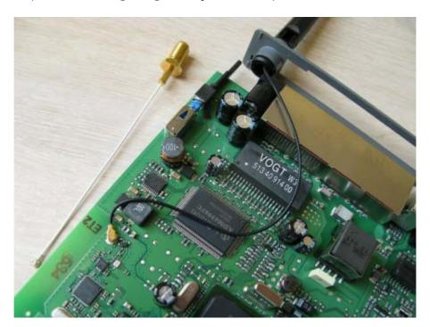
After you open the case, this is what you see. The backplate easily comes loose after you open the enclosure. The antenna sits in a plastic tube in the rear side. The new chassis-connector and cable combo lies beside the case.
