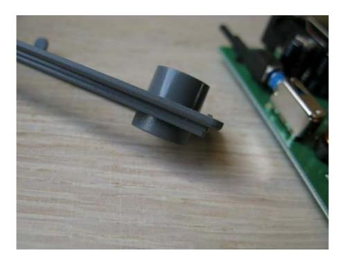
Take a close look at the rear panel. Old antenna is removed. You need to modify the plastic rear panel, in order to place the new SMA antenna connector. The bus, in which the old antenna was held, needs to be cleared!
