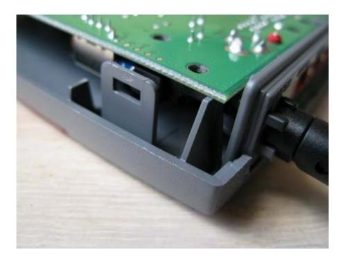
Let's start with the actual modification. It is very easy to open the Fritz!Box. There are four clips, no srews. With a small srewdriver just push the clips sideways. Be careful. If you perform the right movement, the enclosure opens very smoothly. Also, closing it again is just as simple.
