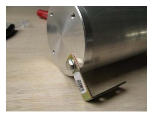
As you can see, there are four mounting holes on the backside of the antenna. This gives you the possibility to radiate your W-LAN signals either horizontally or vertically. If you use only one screw in the bracket, you can play with antenna pointing direction for the best results!
