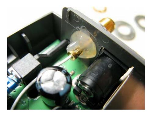
Detailed view of inside backpanel with new connector.
