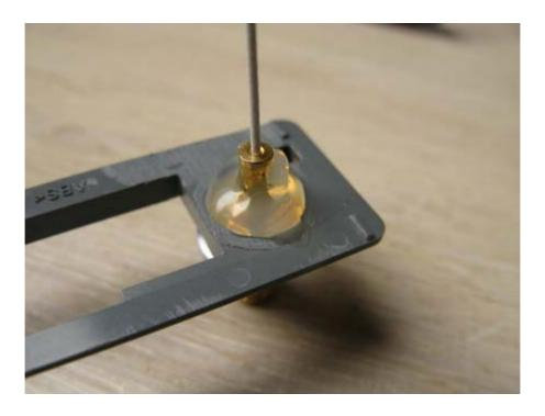
After cooling down, you can click the new printconnector in place on the prinboard.
