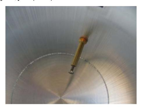
Take a look into the antenna cavity. The metal pin is the actual antenna. With the screw the antenna is tuned to the right frequency. Johannes provides measuring reports for each individual antenna. The can around the antenna put the signals in the right direction and adds to the antenna gain. With the screwholes in the backside you can choose either for horizontal or vertical polarisation.
