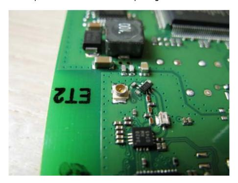
Now, carefully remove the thin coax connector from the printboard. Now, the old fixed antenna is free and can be removed.
